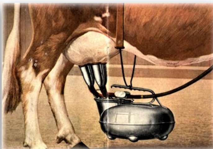
1923 – Pine Tree Surge Milker showing the milker in operation. (Photo credit: www.surgemilker.com )
